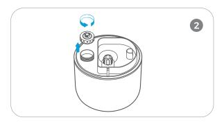
Remove the nozzle, use the handle to remove Water Tank from the base and turn upside down. Remove Water Tank Cap by turning counterclockwise (left).
