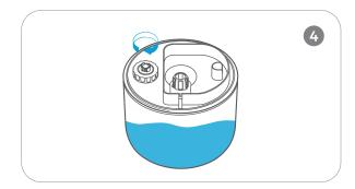
Lock Water Tank Cap by turning clockwise (right).
