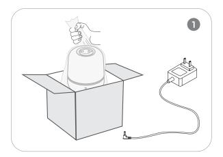
Remove all packaging materials. Remove twist tie from power cord and extend power cord to full length.
