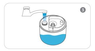
Fill Tank with cool water. **DO NOT** fill with warm or hot water.
