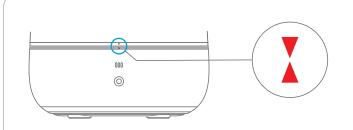
Place Tank on Base. The triangle arrow marks on the side should perfectly align with each other when placement is correct. Water will drain from the Tank into the Base Water Chamber when the Plunger is engaged.
